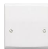
S5045 WHI 45A Cooker connection unit with 3 terminal block, each of which will accommodate up to two nos. of 6mm² conductor
