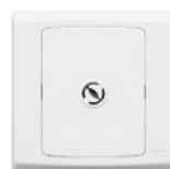
S1090 WHI 25A front flex outlet with 3 terminal block, each of which will accommodate up to 2nos. of 4mm² conductors
